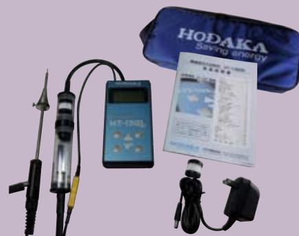
HT-1300Z type A O<sub>2</sub> CO NO<sub>x</sub> °C
